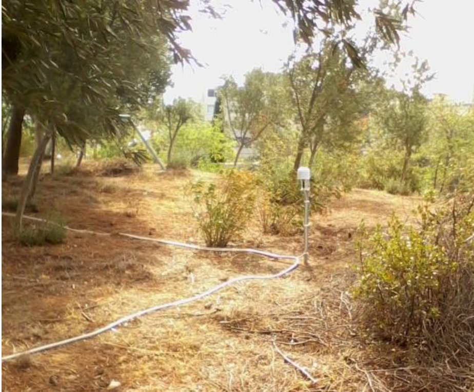
Figure 48. Temperature sensor A2 on the area with natural vegetation.
